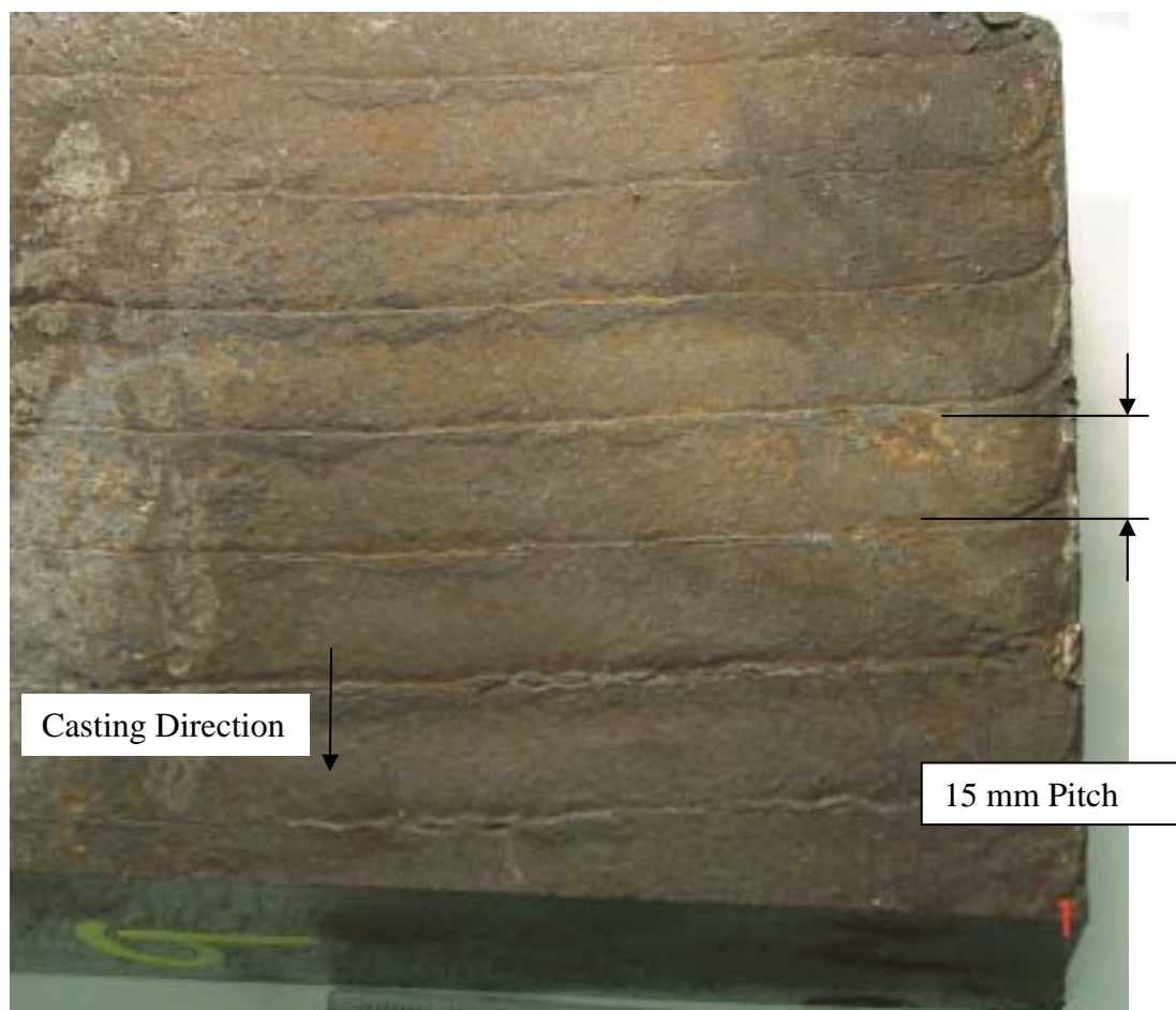
Figure 5.11: Oscillation mark appearance on a slab 114376-06. Marks are measured peak-to-trough and compared to nailboard standing wave measurements. The troughs of the above oscillation marks are not visible due to sample size.
